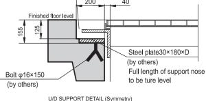
Position of intermediate support is at center of span
